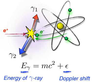
**Fig. 1:** Positrons annihilate with electrons in atoms producing two detectable  $\gamma$ -rays whose energies are Doppler shifted by an amount characteristic of the electron state involved. Positron annihilation is a unique probe for material characterisation, medical imaging and astrophysics.
