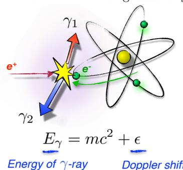
**Fig. 1:** Positrons annihilate with electrons in atoms producing two detectable  $\gamma$ -rays whose energies are Doppler shifted by an amount characteristic of the electron state involved. Positron annihilation is a unique probe for material characterisation, medical imaging and astrophysics.
