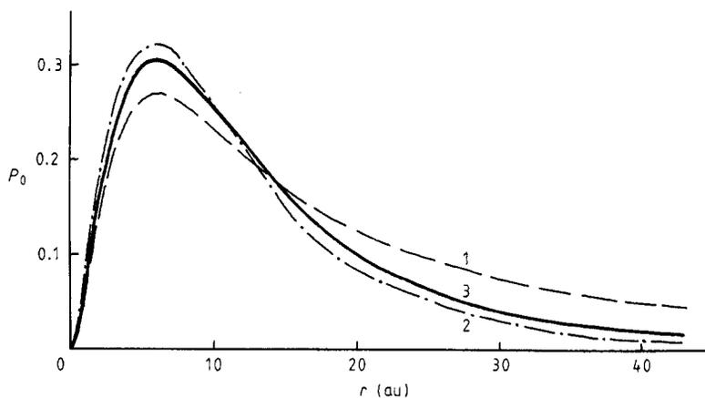
**Figure 2.** Radial 2p-electron wavefunction in  $\text{He}^- 1s2s2p^4P$ : 1, with main self-energy diagram (12a) taken into account ( $\epsilon_0 = -0.0004$  Ryd); 2, with three diagrams (12a-c) taken into account ( $\epsilon_0 = -0.0095$  Ryd); 3, with five diagrams (12a-e) taken into account ( $\epsilon_0 = -0.0062$  Ryd).
