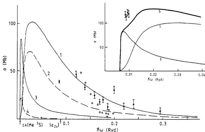
Figure 3. Photodetachment cross sections for  $\text{He}^- 1s2s2p^4P$ . Calculation: 1,  $2p \rightarrow \epsilon d$  channel,  $r$ -form; 2,  $\nabla$ -form; 3,  $2p \rightarrow \epsilon s$  channel,  $r$ -form; 4,  $\nabla$ -form; 5, total  $2p$ -photodetachment cross section,  $r$ -form. Experiment:  $\circ$ , Compton *et al* (1980);  $\bullet$ , Hodges *et al* (1981).
