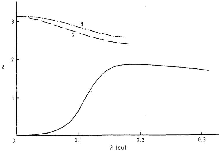
**Figure 1.** The  $p$  phaseshift for electron quartet scattering by He  $1s2s^3S$ : curve 1, Hartree-Fock approximation; 2, with main self-energy diagram (12a) taken into account; 3, with three diagrams (12a-c) taken into account.
